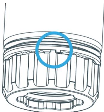
2. Push the ratchet plate against the spring and turn the nut over the stop. You can use a flat blade screwdriver for this. Now you can rotate the nut another turn. Repeat this step until the nut comes off the suppressor.
